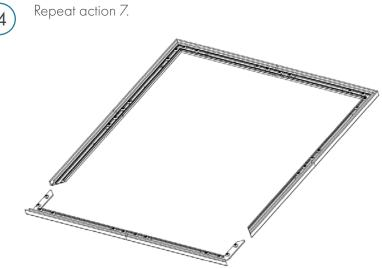
Holes within the frame are for mounting your SEG Tension Frame to a wall. Maximum distance between holes is 500mm.
